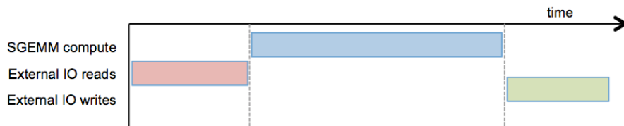
Figure 7 When the data initially resides in the external memory, the data is first transferred into local memory before computation starts. The result data can be written back to external memory once completed.
